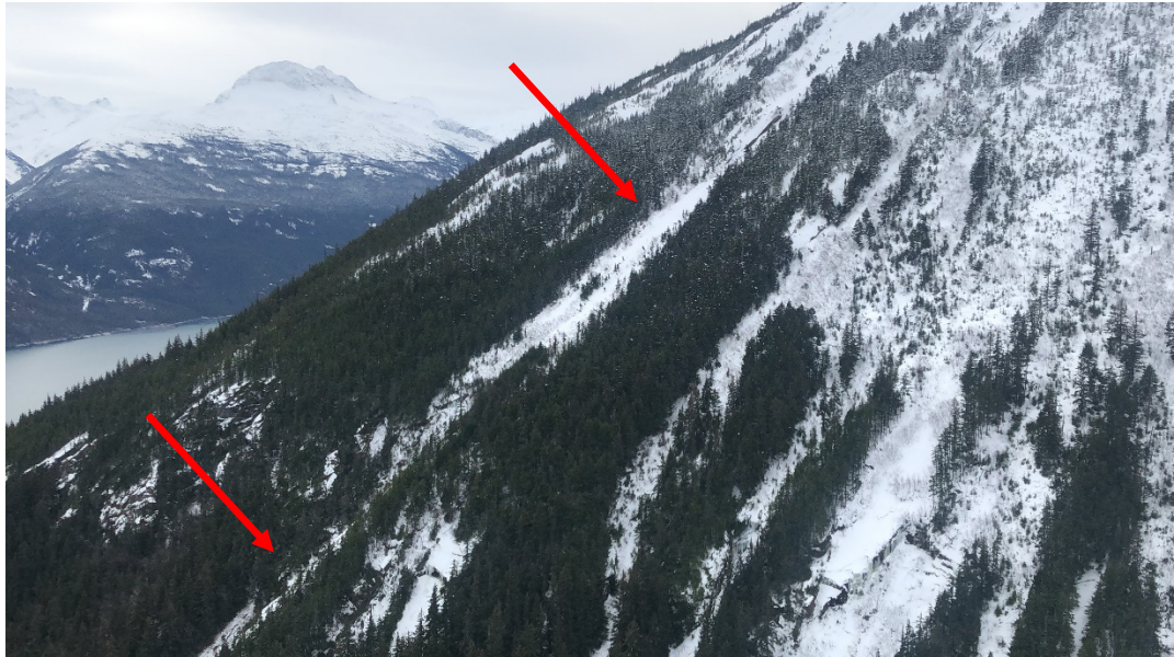
Photo looking southeast at slopes immediately west of the slide, which is not visible in this photo. Red arrows point to a rock structure-controlled linear feature (similar to the features above the landslide discussed in this report) that appears to channelize flow of water and debris to valley bottom. The termination of this feature is approximately 2,500 feet upstream of the property line at Burro Creek and approximately 3,000 feet upstream of the landslide discussed in this letter.
